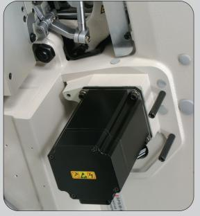
① Having been applied with the SunStar direct drive system, the main machine's responsiveness and the ability to stop accurately. It provides are used to link the AC motor to the upper shaft, improving the optimal conditions to produce high-quality sewing products. body of the sewing machine is directly attached to the motor. Couplings
